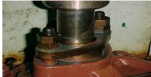
Gambar 1. 3 Stuffing Box pompa sentrifugal
