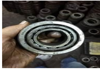
Gambar 1. 13 Van Bearing & Ball Bearing pompa sentrifugal
